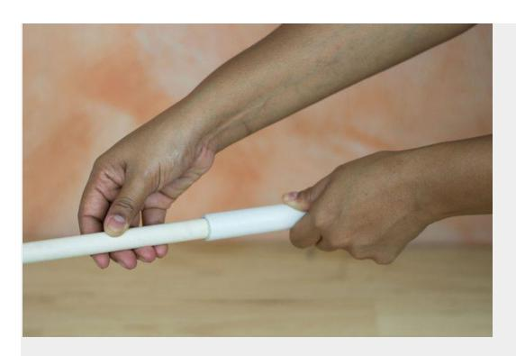
Ensure that the smaller pipe fits inside the larger pipe. It should slide and not be tight, but it should not wobble. If it does not slide smoothly inside the larger pipe, use an even smaller-diameter pipe.
