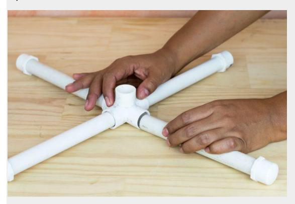
Insert four 2-foot PVC pipes into a five-way cross connector so that they form a foot for the pole. Slide an end cap on each pipe.
