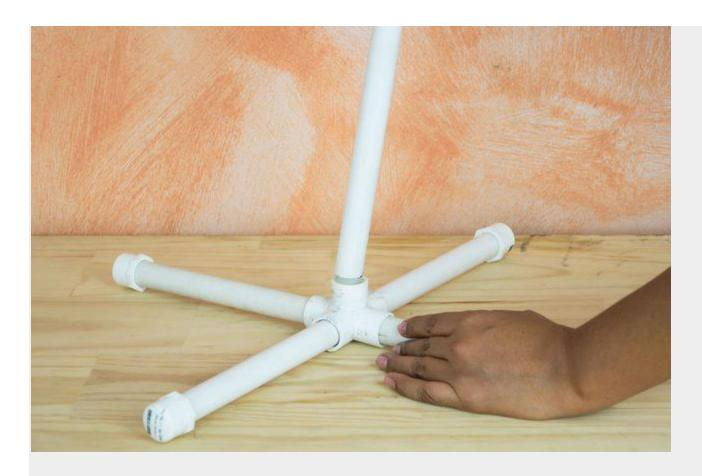
Insert the larger pipe you drilled into the fifth hole of the cross connector. Slide the smaller pipe inside and secure the height with the ringed pin. The telescoping pole is now finished.
