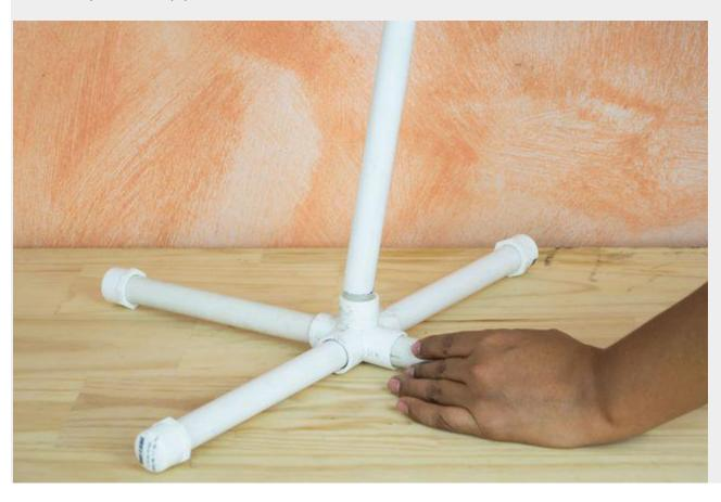
Insert the larger pipe you drilled into the fifth hole of the cross connector. Slide the smaller pipe inside and secure the height with the ringed pin. The telescoping pole is now finished.
