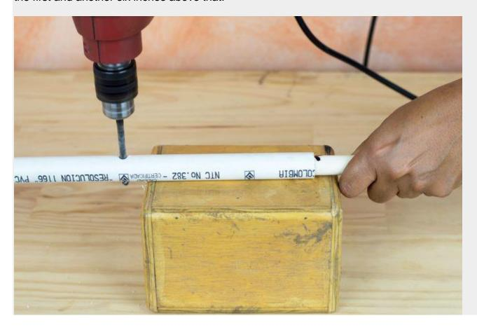
Slide the smaller pole inside the larger one. Line up the first X on the smaller pipe with the hole you drilled in the larger one. Holding it firmly, drill through the smaller pipe while it is inside the larger one. The drilled holes should line up and allow you to insert the ringed pin all the way through both pipes.
