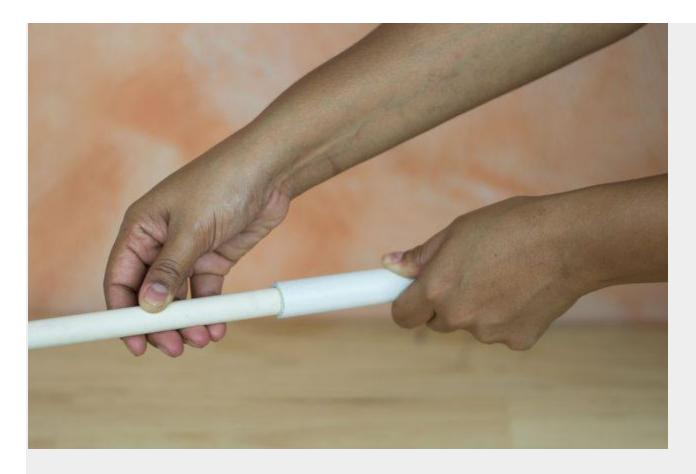
Ensure that the smaller pipe fits inside the larger pipe. It should slide and not be tight, but it should not wobble. If it does not slide smoothly inside the larger pipe, use an even smaller-diameter pipe.
